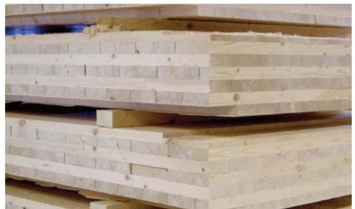
Figure 1: Stacked CLT Panels [6]
